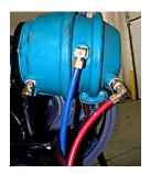
Roto-Chamber – uncommon brake type. Identified by a series of fasteners around the outer circumference of the chamber.
