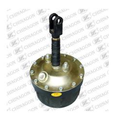
DD3 – (Double Diaphragm, 3 function) – typically found on MCI highway coaches. Identified by three air fittings.
