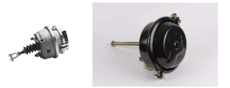
Bolt – uncommon brake chamber. Identified by a series of bolts securing the cap to the body of the chamber.
