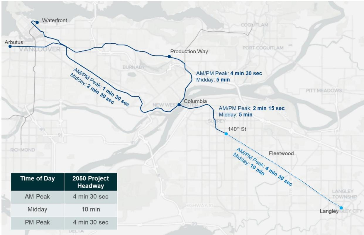
Figure 4-5 compares the Project extension’s practical capacity in passengers per hour per direction (pphd) to the Canada Line and Evergreen Line. By 2050 the Project will be able to carry approximately 7,560 passengers per hour per direction (pphd) during the AM / PM peak, and 3,400 pphpd during off-peak hours.
