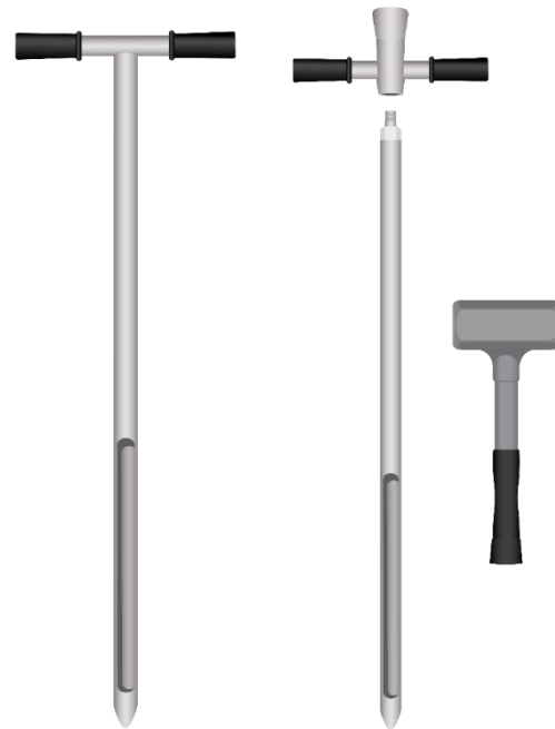
Figure 1. Examples of soil sampling equipment: a soil push probe and a soil hammer probe.
