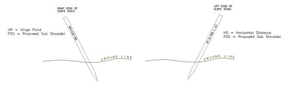
The stake is set at a  $\pm 30^{\circ}$  to  $\pm 40^{\circ}$  degree angle with the front face of the stake facing centerline, and the station indicated on the back.
