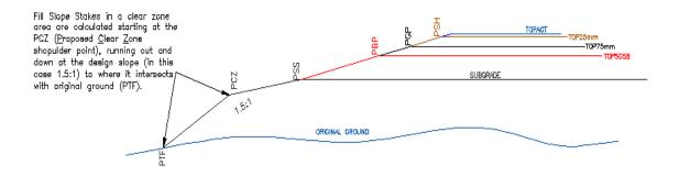
**Example 3: Proposed Top of Cut (PTC)** and probable slope stake location scenario from a CAiCE cross-section template EAR file in a Type-D excavation.
