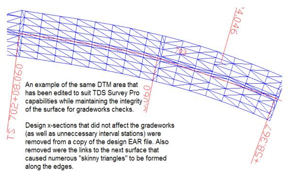
Example of functional, edited, design grade DTM in TDS Survey Pro software on a Recon Survey Data Collector
