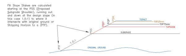
**Example 2: Proposed Clear Zone (PCZ)** and probable slope stake location scenario from a CAiCE cross-section template EAR file (once the fill has reached the PCZ hinge point, another slope stake calculated from the PSS on differing slopes may be required)
