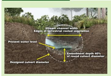
The two diagrams depict a culvert cross section projected on a natural stream channel. It is critical that the design culvert width is as wide or wider than the natural stream channel to be a successful streambed simulation.
