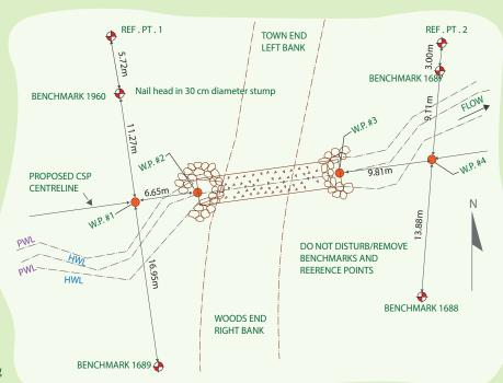
Clearly mark reference points and benchmarks in the field and describe them on design drawings. For example, "nail head in 30 cm diameter stump."
