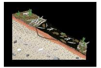
3. Replace topsoil\duff and place slash on top, similar to surrounding cut block.
