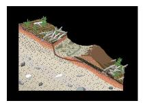
1. Remove woody debris from running surface and decompact in an outsloping manner.
