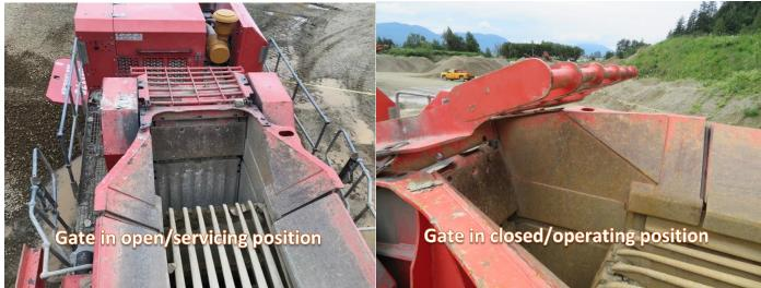
When the safety gate is not securely attached with bolts in its operating position, it can be dislodged by rocks forcefully rejected by the jaw.
