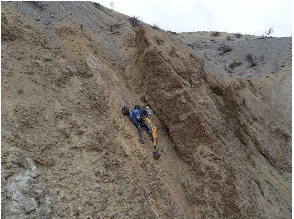
The spider excavator starting its descent down the west bank on Sept. 19, 2019.
