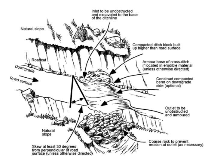
A well-compacted ditch block will be installed immediately downgrade of the cross-ditch inlet. The ditch block is usually higher than the road surface. The ditch block should be non-erodible, relatively impermeable, and large enough to divert all expected flows into the cross-ditch. Where ditchwater converges at low points in the road, no ditch block or berm is required, as the cross-ditch should be constructed as a broad gentle swale.
