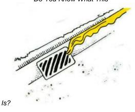
This is called a 'storm drain' or 'catchbasin'. There are many of these drains located throughout your neighbourhood. Their purpose is to collect rain and melted snow that drain off exposed surfaces such as roads, parking lots and driveways.
