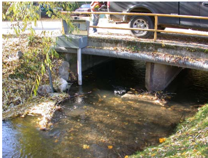
Figure C-10. The deployment tube must protect the sensors from debris, such as leaves and branches, in the stream. Photo: Linda Gregory
