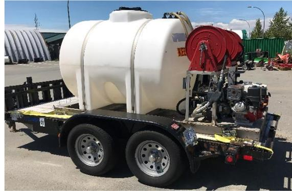
**Figure 9b.** Truck mounted pressurized sprayer used for pesticide applications.
