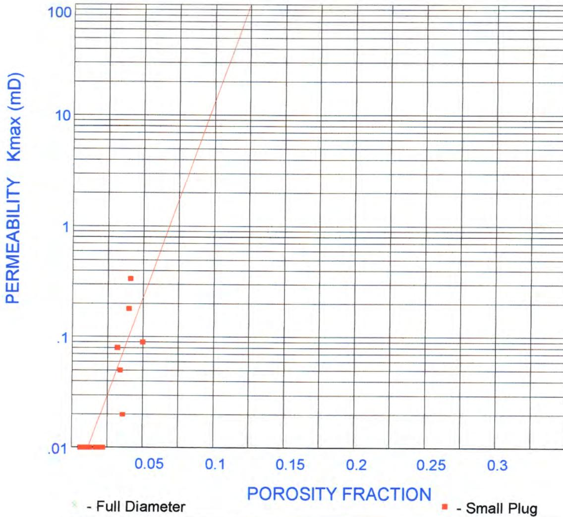
Equation of Line :  $\text{Log (Kmax)} = -2.41 + 35.29 * \text{Porosity}$
