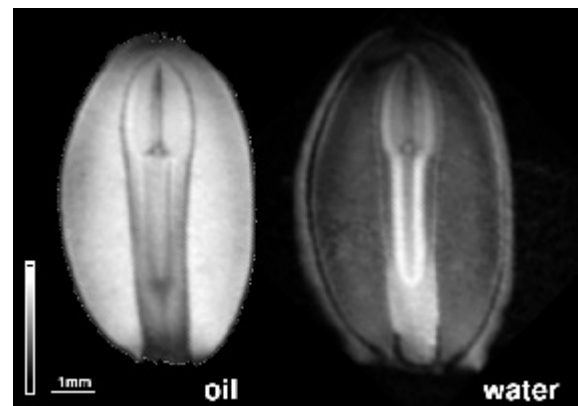
Figure 3. MRI images for oil and water recorded simultaneously in the same imbibed Ponderosa pine seed.
