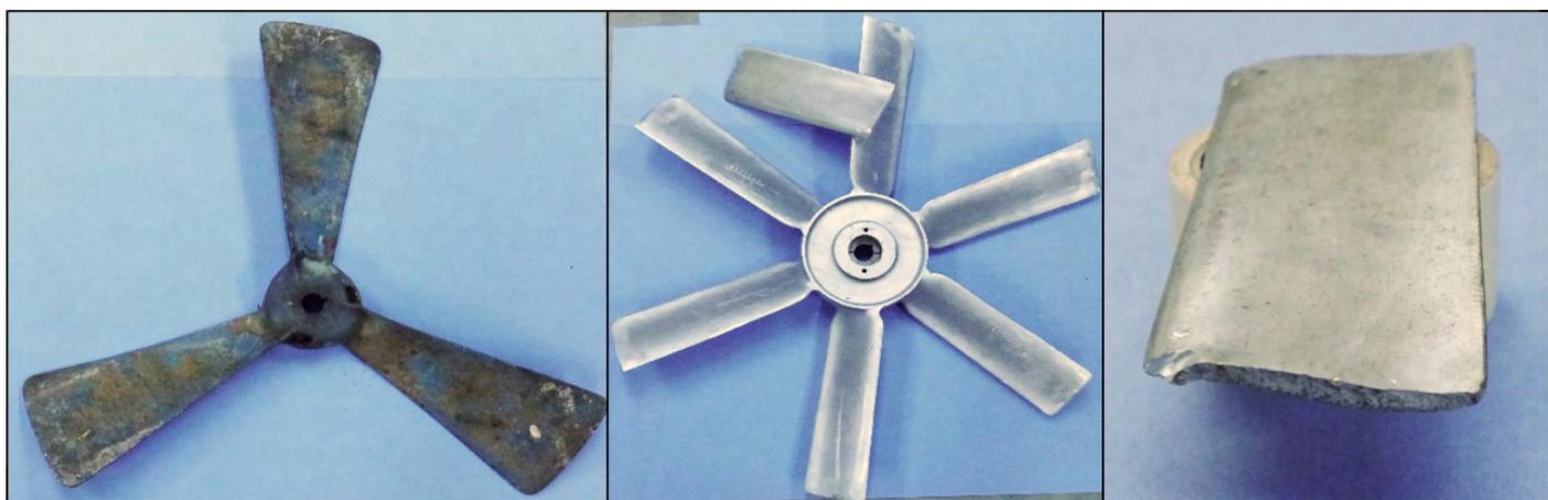
Figure 3. Kiln fans: the old, the new, and the broken blade.
