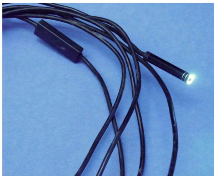
Figure 6. Endoscope used to observe cone opening.
