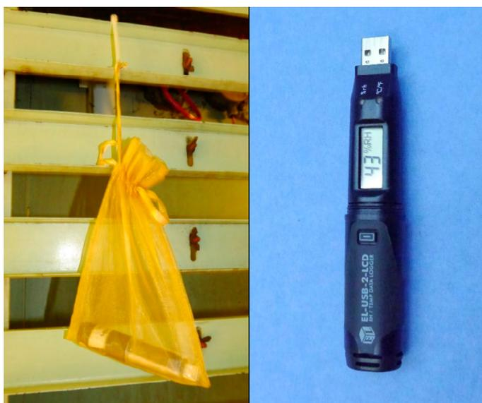
Figure 2. A downloadable temperature and RH% data logger placed inside the kiln.
