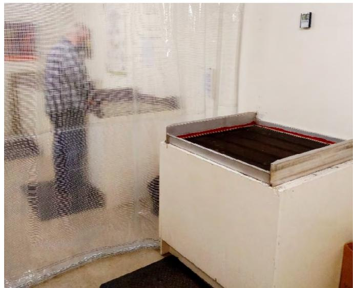
Figure 2. The surface drying tables used at the BC Tree Seed Centre. The clear curtain is used to separate the two technicians, for COVID-19 safety, who generally will each be managing two drying tables.
