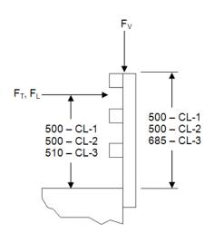
Figure 3-1 Minimum Bridge Barrier Height and Load Application Height
