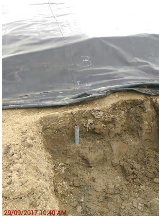
Photo 1.6 – Clay sample being collected with a Shelby tube in test pit #3.
