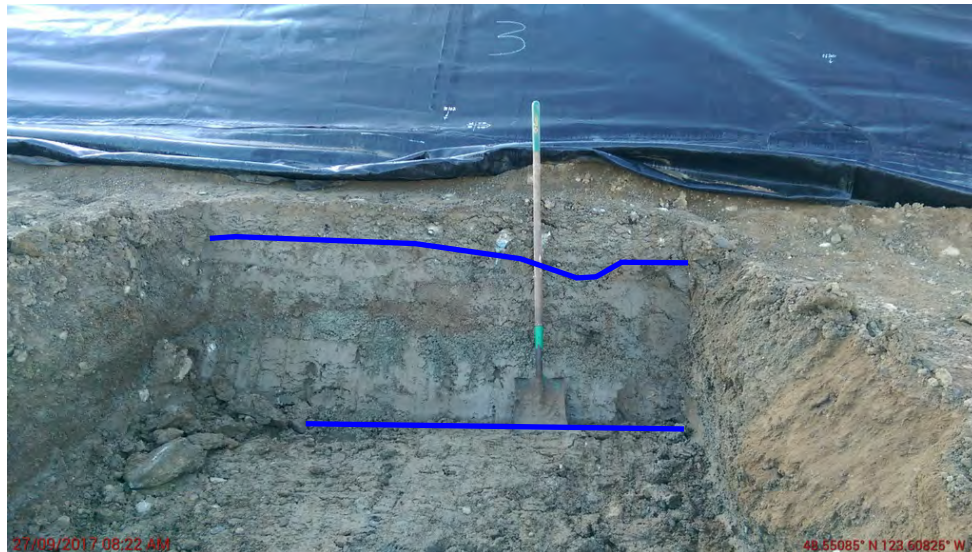
Photo 1.3 – Clay observed in Test pit #3. Blue lines represent top and bottom of observed clay layer.
