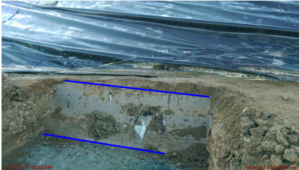
Photo 1.1 – Clay observed in Test pit #1. Blue lines represent top and bottom of observed clay layer.
