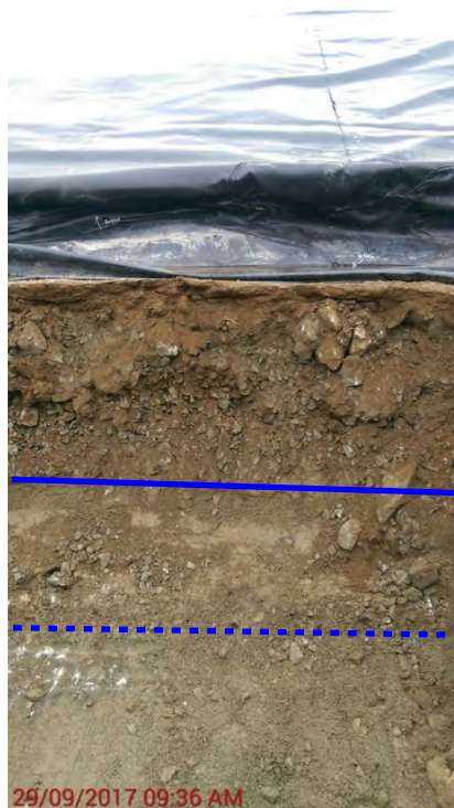
Photo 1.4 – Clay observed in additional test pit located 10 metres west of test pit #3. Blue solid line represents top of observed clay layer. Dashed line represents base of excavation; the presence of clay below the dashed line was undefined.
