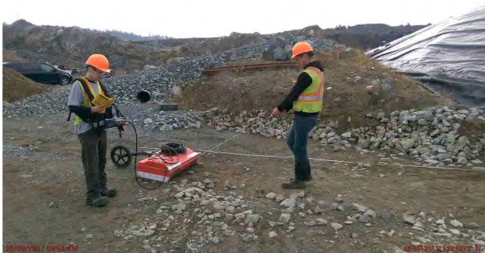
Photo 1.7 – Frontier calibrating their GPR instrument.
