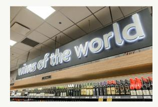
The LDB designed a new type of light emitting diode (LED) perimeter signage. In remodeled locations, this type of signage replaced less efficient neon signs.
