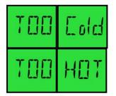
Device temperature **TOO Cold** for test type being performed.
