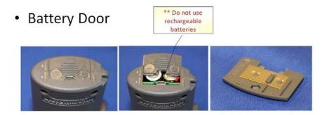
**Batteries** - The battery cover is located on the base of the Alco-Sensor FST®. Two AA alkaline batteries should run well in excess of 1000 tests at room temperature. The device is reverse-polarity protected. Rechargeable batteries are not to be used.
