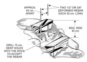
TREADS SHALL BE SHAPED AND PLACED OVER REBARS TO PROVIDE A FIRM, SOLID CONTACT WITH THE ROCK AND SHOULD BE APPROXIMATELY LEVEL OR SLIGHTLY IN TOWARDS THE ROCK
