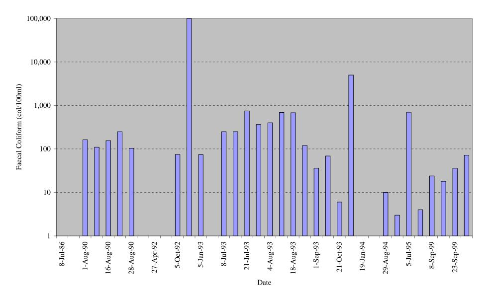
Figure 5.13 Faecal Coliform Concentrations in the Fruitvale STP Effluent from 1986 to 1999
