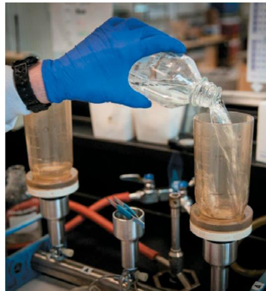
Rinsing the filter housing for membrane filtration.
