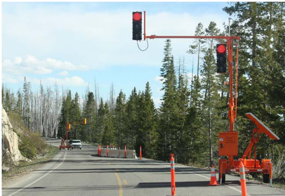
Figure 4.21: Portable Traffic Signal Mounted on Trailer
