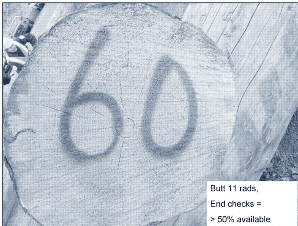
Figure 3: Photo of log with end checks used in a training presentation relating to the Scaling Requirements (Ex. C-84, at CAN-010314)
