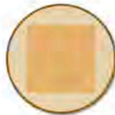
Figure 1B. Illustration B of a log with 49 percent of its volume available to manufacture lumber
