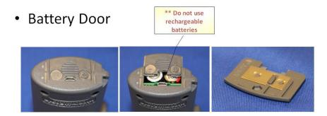
**Batteries** - The battery cover is located on the base of the Alco-Sensor FST<sup>®</sup>. Two AA alkaline batteries should run well in excess of 1000 tests at room temperature. The device is reverse-polarity protected. Rechargeable batteries are not to be used.
