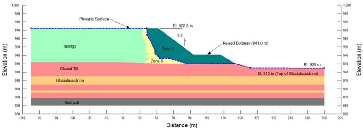
**Figure 4.18** KCB Stability Model Set-Up – Section D – Crest Elevation 972.5 m w/ Buttress
