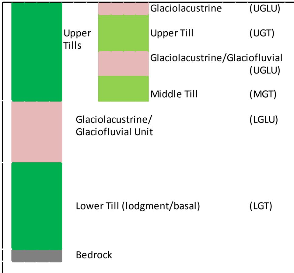
**Figure 4.1 Schematic of Generalized Soil Units**
