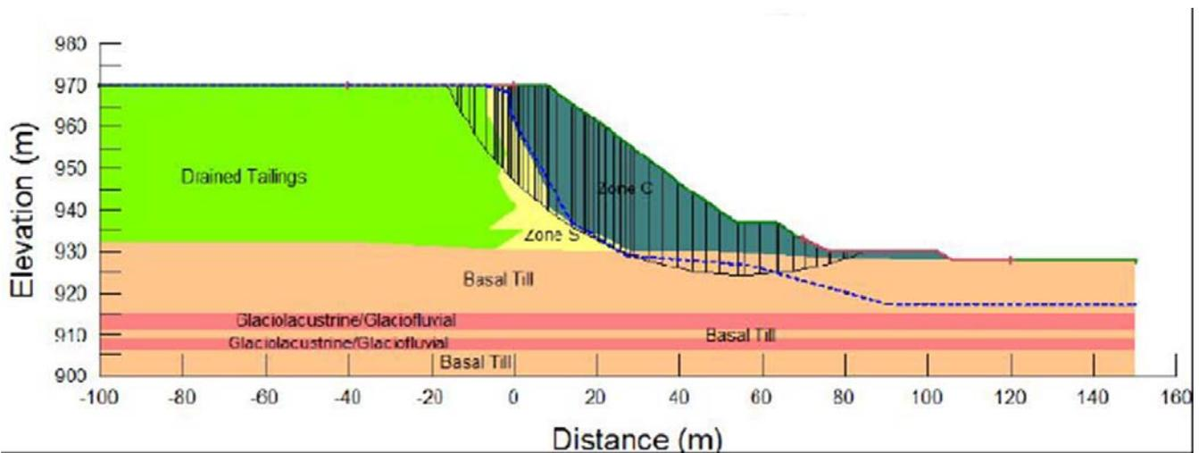
**Figure 3.7** AMEC Geologic Model used for Stability Analysis of Stage 9 Perimeter Embankment (3+990, Section D) (AMEC 2013b)
