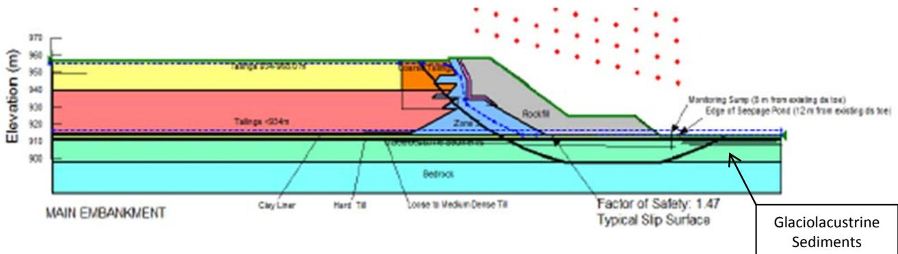
**Figure 3.4 KP Geologic Model for the Main Embankment used for Stage 6 Report (KP 2014)**
