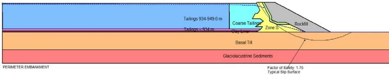
**Figure 3.5 KP Geologic Model for the Perimeter Embankment used for Stage 6 Report (KP 2014)**
