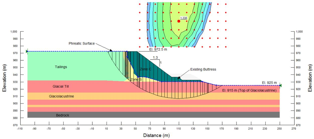
**Figure 4.19 KCB Stability Model –Typical Critical Slip Surface with Peak GLU Strength**
