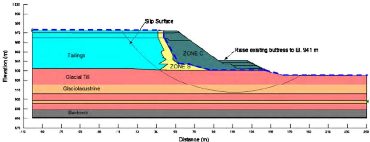
**Figure 3.9 BGC Geologic Model used for Stability Analysis of Stage 10 Perimeter Embankment (3+990, Section D) (BGC 2014)**
