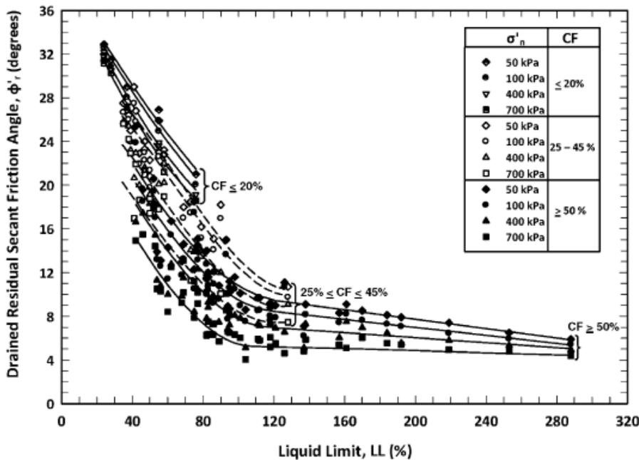
**Figure 4.10 Correlation between Residual Friction Angle and Liquid Limit (from Stark and Hussain 2013)**
