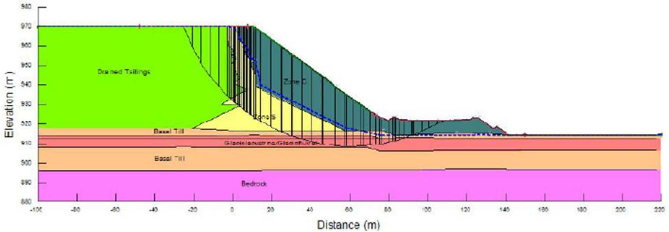
**Figure 3.6** AMEC Geologic Model used for Stability Analysis of Stage 9 Main Embankment (1+850) (AMEC 2013b)
