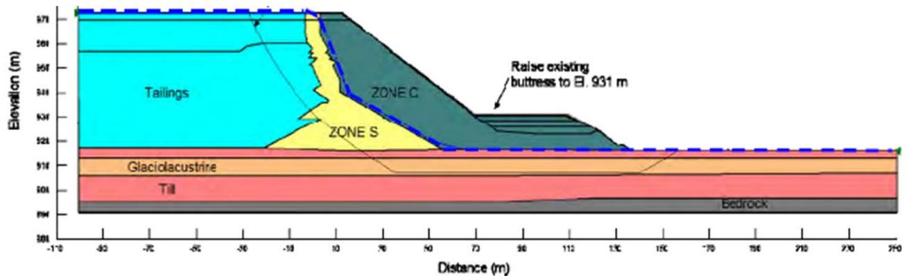
**Figure 3.8 BGC Geologic Model used for Stability Analysis of Stage 10 Main Embankment (1+900) (BGC 2014)**
