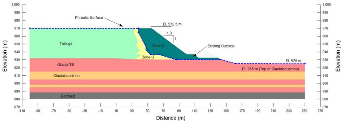
**Figure 4.17** KCB Stability Model Set-Up – Section D – Crest Elevation 972.5 m no Buttress
