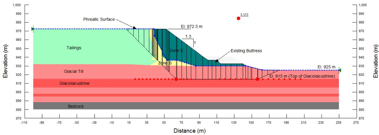
**Figure 4.20 KCB Stability Model –Typical Critical Slip Surface with Residual GLU Strength**
