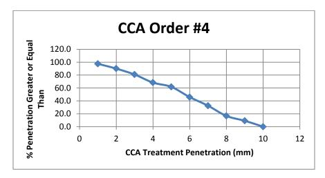
The data for all of the remaining orders (9) were collated into a single data set of (428 measurements) and the frequency of depth of penetration plotted against depth of penetration. This was done to compare against requirements of CSA 080 which specifies a required percentage of penetration exceedance.
