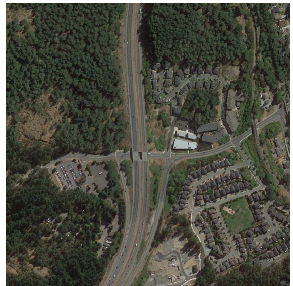
An example of a half diamond interchange. A half diamond is used where traffic patterns require a connection in one direction only, or as a supplement to a nearby interchange.
