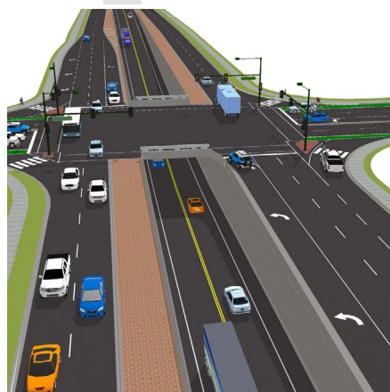
Example of a median express lane. At crossings, the express lanes go under the cross street and the remaining four lanes would be signalized.
