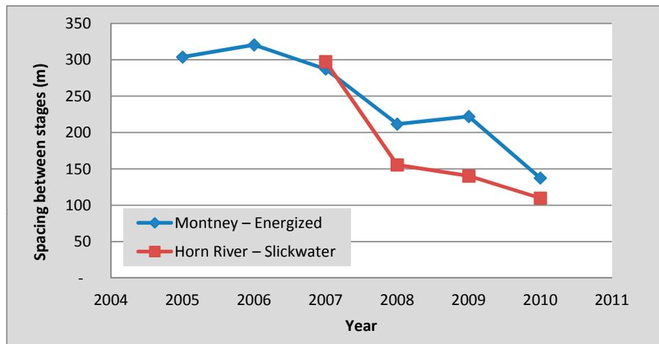
Figure 8. Changes in the average spacing between fracture stages from 2005 to 2010.
