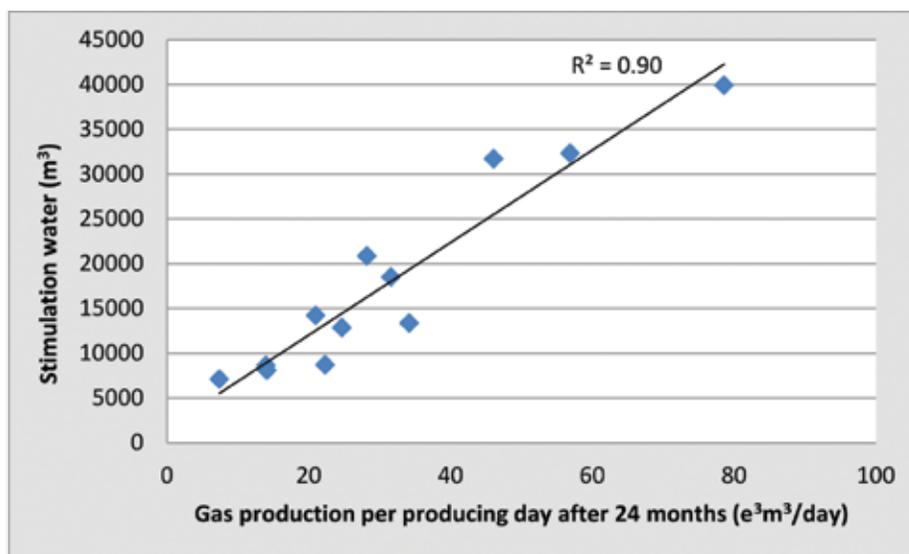
Figure 13. Relationship between stimulation volume for slickwater fractures in the Muskwa–Otter Park formation and later gas production after two years.
