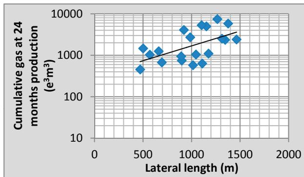
Figure 10. Cumulative gas production after 24 months for wells in the Muskwa-Otter Park shales in the Horn River Basin.
