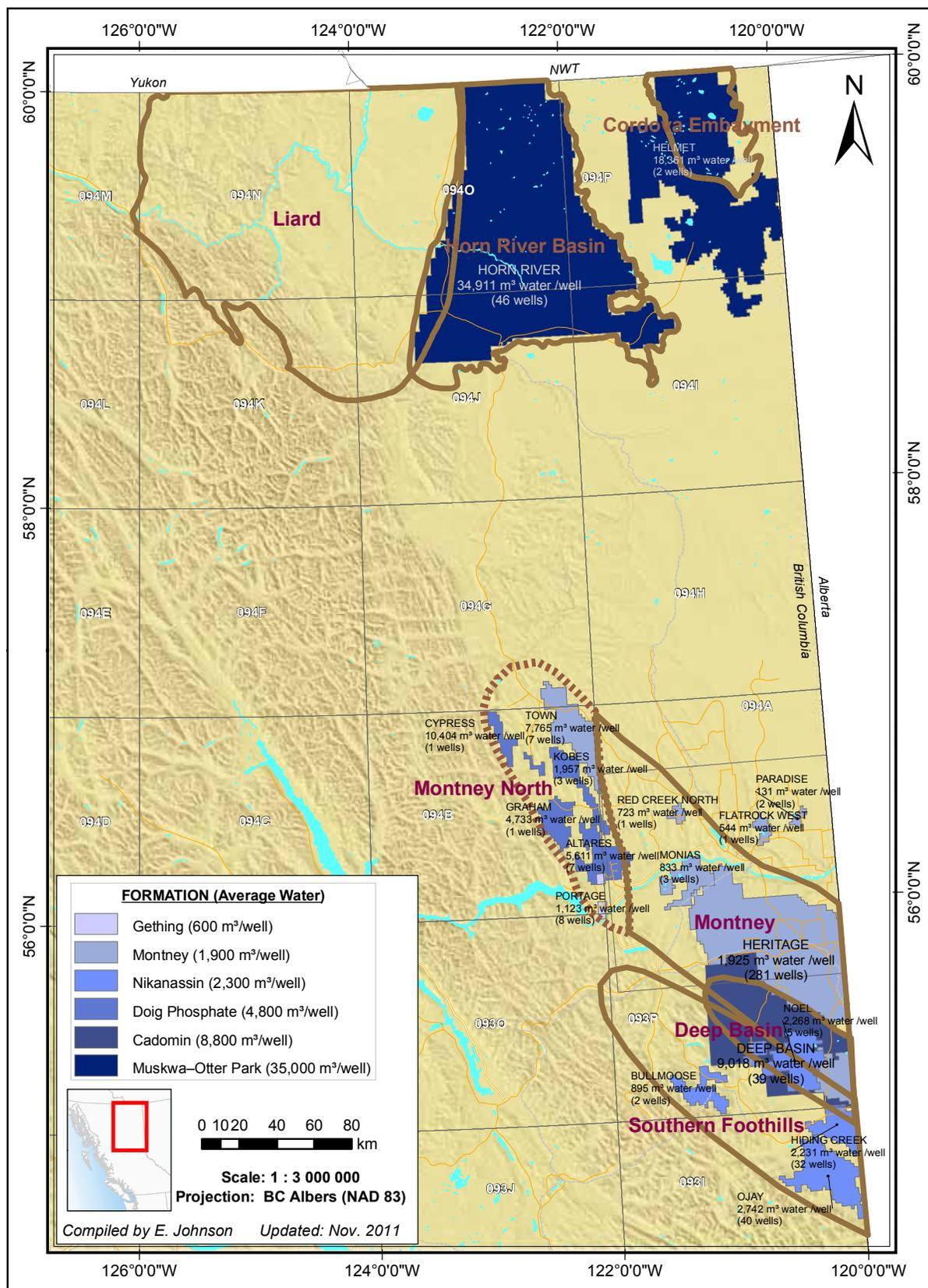
Figure 17. The formations being targeted in the five main basins. The water usage per well has been averaged by multistage wells in that formation and is represented by colours grading from light blue (lowest) to dark blue (highest).
