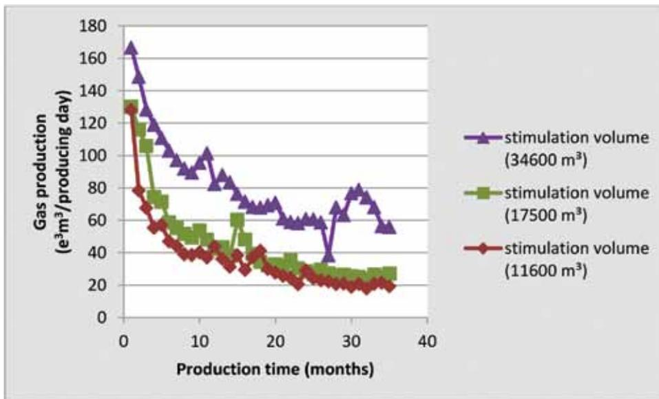
Figure 14. Representative production decline curves in the Muskwa–Otter Park shales for different stimulation volumes. Production curves are grouped according to the initial stimulation volumes as 11 600 m<sup>3</sup>, 17 500 m<sup>3</sup> and 34 600 m<sup>3</sup>, respectively.
