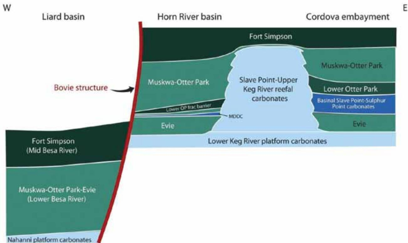
Figure 2. Illustrated cross section depicting shale of the Horn River Basin and the Cordova Embayment separated by the Presqu'île barrier reef (Ministry of Energy and Mines and National Energy Board, 2011).
