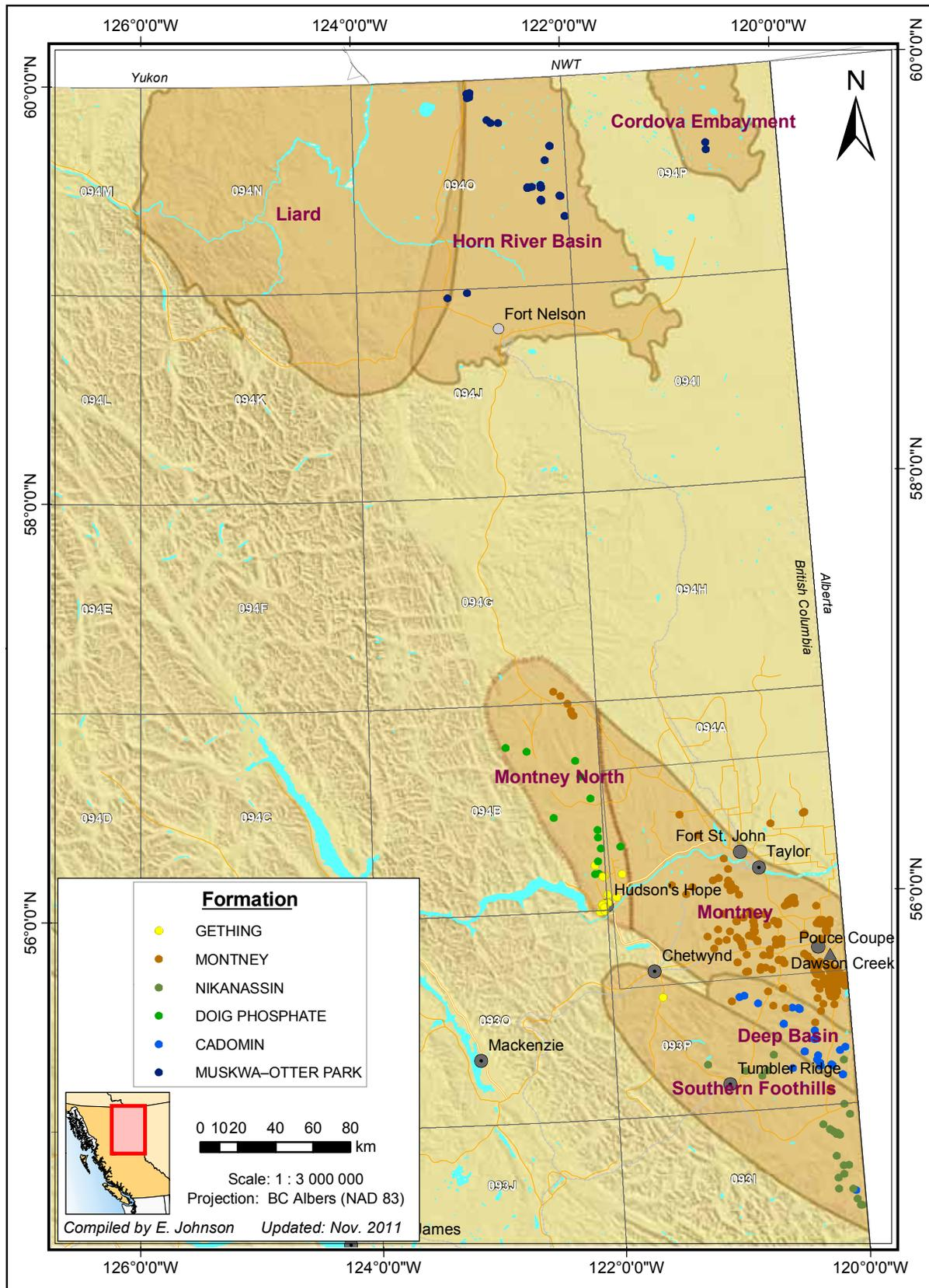
Figure 1. Major basins with multistage fracturing in northeast British Columbia. Wells are indicated as solid dots and formations are grouped by colour.
