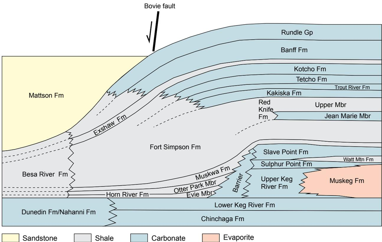
Figure 3. Schematic diagram shows the transition (in grey) between the Besa River Formation in the Liard Basin (left) to the package in the Horn River Basin (right), which ranges from the Evie, Muskwa–Otter Park members through the Debolt Formation (Ferri et al., 2011).
