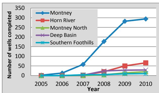
Figure 4. Development activity showing the well count for multi-stage wells in northeast British Columbia by basin.
