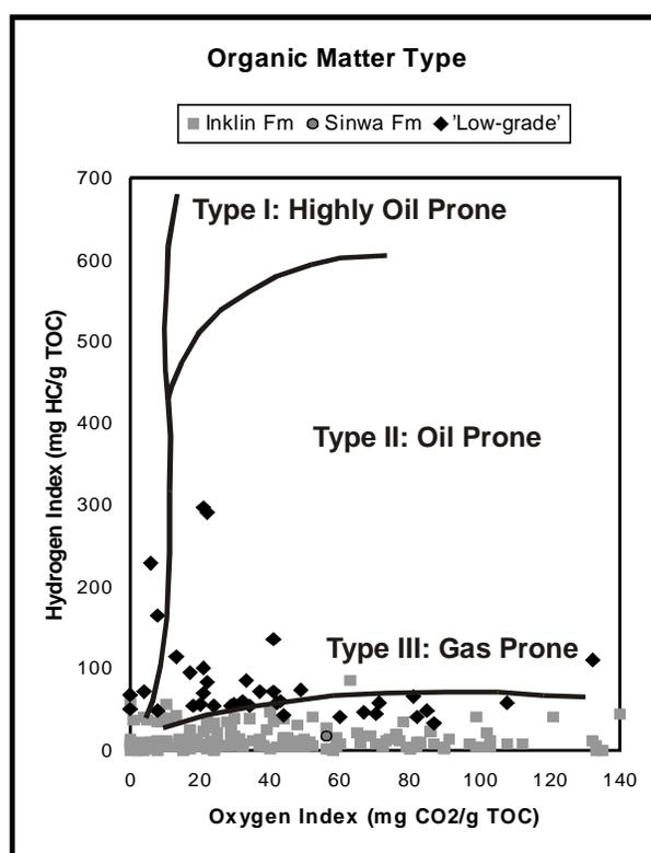
Figure 4. Plot of hydrogen index versus oxygen index for samples from the central Whitehorse Trough. 'Low-grade' samples form a subset of the Inklin Formation samples, for which  $S_2 > 0.2$  and  $T_{max} < 480$  °C. The organic matter type in a source rock can be determined from this plot (Espitalié et al., 1977).
