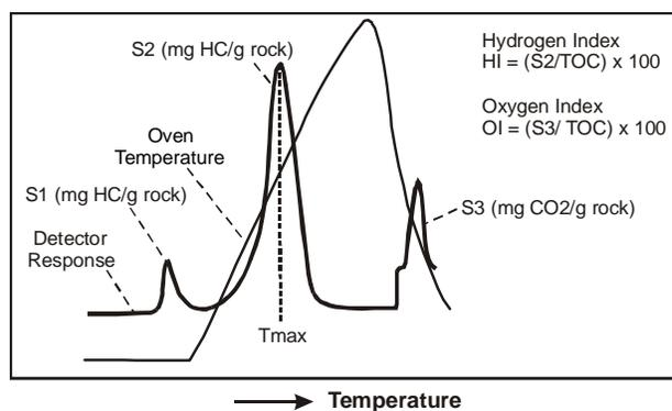
Figure 2. Schematic pyrogram illustrating the liberation of hydrocarbon during heating of the rock sample. Determined parameters include  $S_1$ ,  $S_2$ ,  $S_3$ ,  $T_{max}$ , and the hydrogen and oxygen indices.
