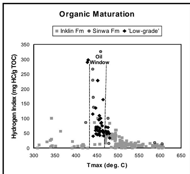
Figure 5. Plot of hydrogen index versus  $T_{max}$  for samples from the central Whitehorse Trough. 'Low-grade' samples form a subset of the Inklin Formation samples, for which  $S_2 > 0.2$  and  $T_{max} < 480$  °C. Due to low  $S_2$  values,  $T_{max}$  values for the majority of other Inklin Formation samples are suspect and are dominantly overmature.
