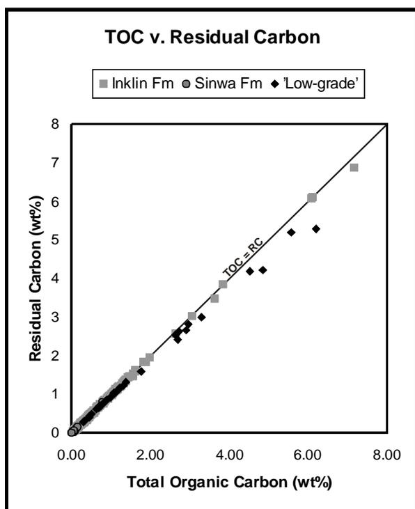
Figure 3. Plot of total organic carbon (TOC) versus residual carbon for samples from the central Whitehorse Trough. 'Low-grade' samples form a subset of the Inklin Formation samples, for which  $S_2 > 0.2$  and  $T_{max} < 480$  °C.
