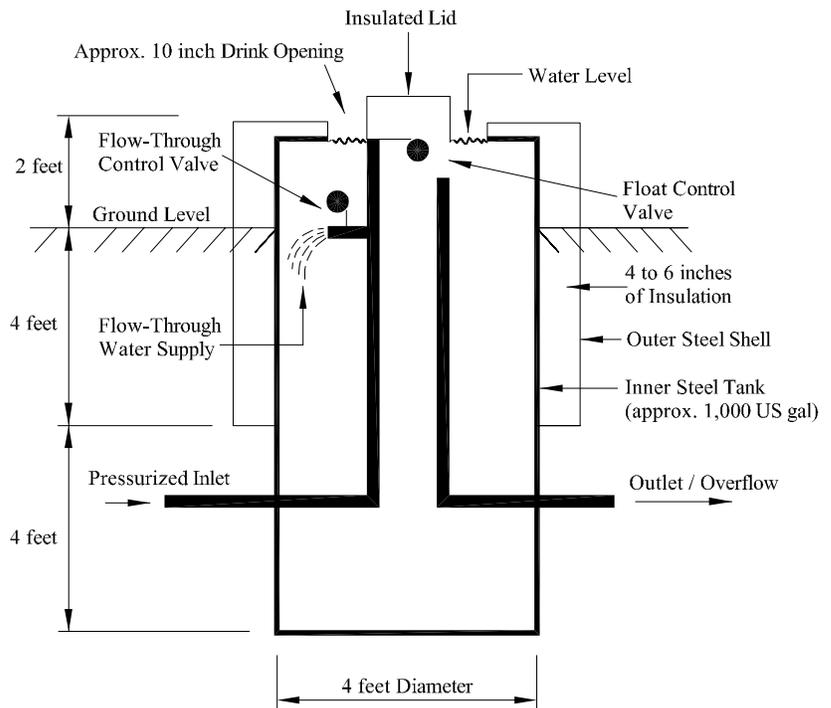
Note this trough has heat supplied with flow-through water combined with wall insulation and small water surface area for reduced heat losses. It may be used as a float controlled waterer or as a flow-through one.
