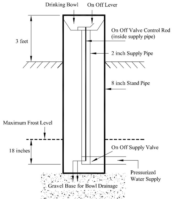
When the lever is off, the supply pipe drains down to the supply valve.
