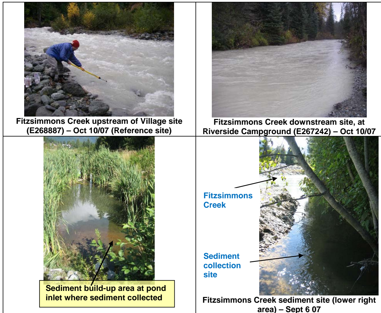
Photo Series 5.2: Fitzsimmons Creek water sampling sites showing upstream and downstream locations (upper row) and sediment sampling locations in biofiltration pond inlet (bottom left) and outlet of the pond discharge mixed with the 'amenities stream' as it enters Fitzsimmons Creek (bottom right)
