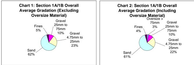
Appendix D provides a plot of the average gradations curves excluding (Chart D1-1) and including (Chart D1-5) the oversize portion. The resulting overall average gradation of the granular materials indicates the soil is gravelly sand with a trace silt and a trace cobbles (up to 200 mm diameter).
