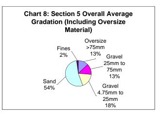
Appendix D provides a plot of the average gradations curves excluding (Chart D5-1) and including (Chart D5-5) the oversize portion. The resulting overall average gradation of the granular materials indicates the soil is a sand and gravel, with a trace to some cobbles and a trace boulders (up to 300 mm diameter).
