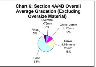
Appendix D provides a plot of the average gradations curves excluding (Chart D4-1) and including (Chart D4-5) the oversize portion. The resulting overall average gradation of the granular materials indicates the soil is a gravelly sand with a trace silt, a trace cobbles and a trace boulders (to 250 mm diameter).
