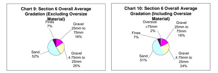
Appendix D provides a plot of the average gradations curves excluding (Chart D6-1) and including (Chart D6-5) the oversize portion. The resulting overall average gradation of the granular materials indicates the soil is a sand and gravel with a trace silt and a trace cobbles.
