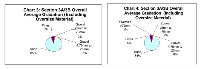
Appendix D provides a plot of the average gradations curves excluding (Chart D3-1) and including (Chart D3-5) the oversize portion. The resulting overall average gradation of the
