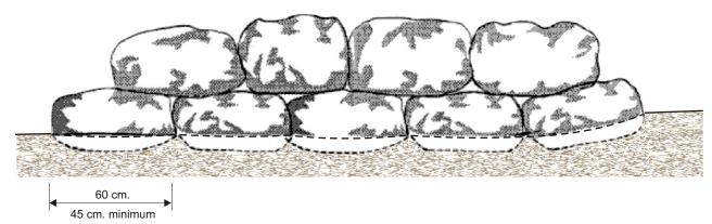
SIZE OF THE BARRIER STONES **SHALL BE** (APPROX.) 35 cm. IN HEIGHT AND WIDTH AND **60 cm. IN LENGTH.**
