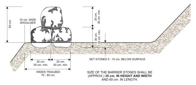
MINIMUM DIMENSIONS **SHALL NOT BE LESS THAN 30 cm. IN HEIGHT AND WIDTH**AND 45 cm. IN LENGTH.
