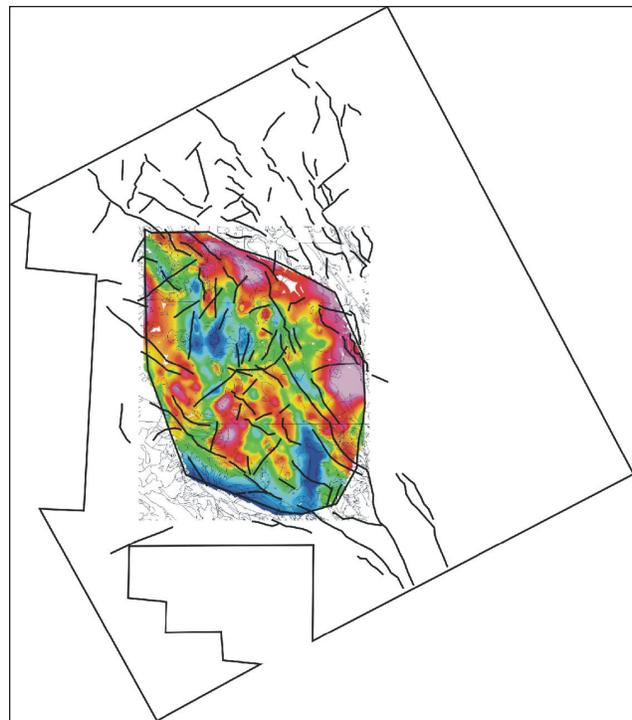
**Figure 8: Bouguer gravity map with geology polygons and lineaments.**
