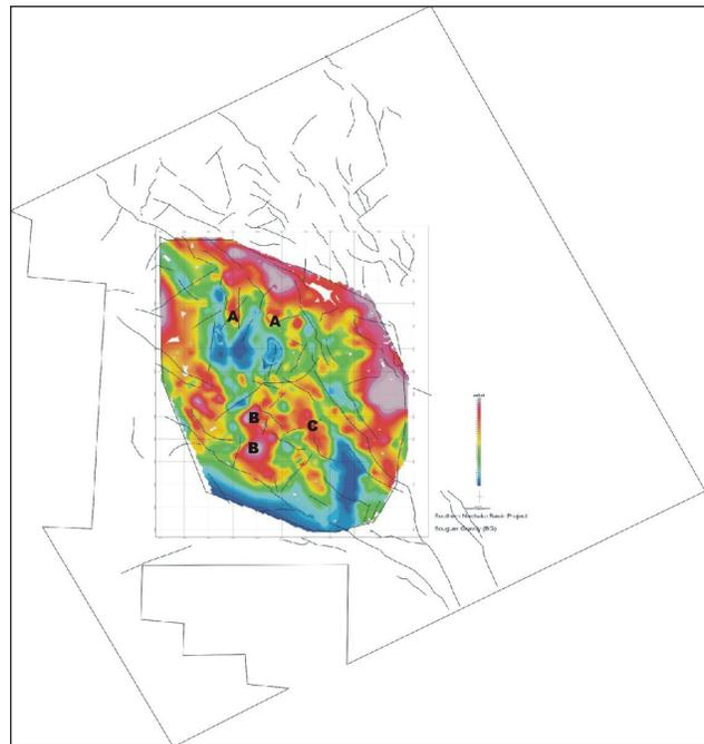
**Figure 7: Bouguer gravity map with lineaments overlain on it.**
