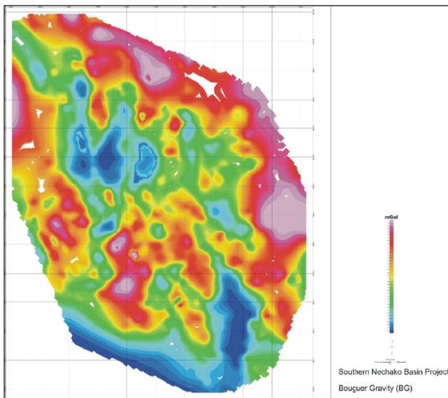
**Figure 2: Bouguer gravity map generated from the digitized contour data.**
