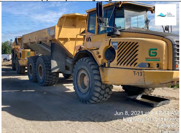
Photo 19. L1170 (F). Parked equipment with spill tray properly in use.
