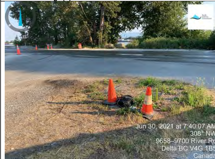
Photo 9. L350 (C). Vibration monitoring for pile driving during guide sign installations.
