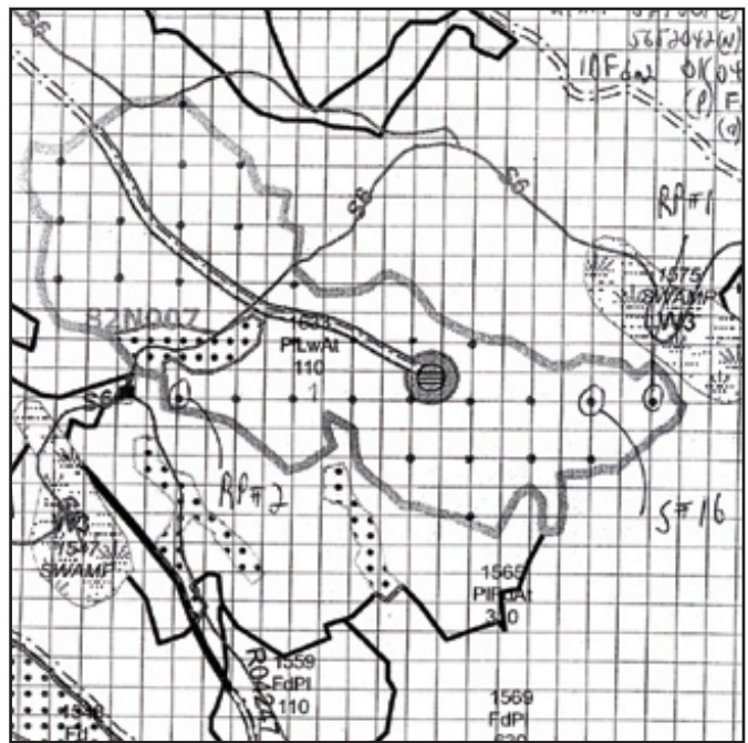
Figure A3-1-B. Example of the sample location process. A uniform grid was photocopied onto the cutblock map. Grid points within the polygon NAR were identified, numbered, and one number selected at random for the sample location. Two additional points were selected at random to serve as replacement points. In the field, crews used the map to determine distance and bearing to the sample point.
