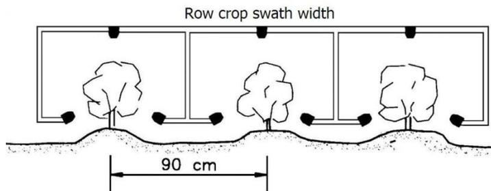
The swath width is used in sprayer calibration to calculate the sprayer's delivery rate. As the sprayer swath width is based on the treated area, the delivery rate will also be based on the treated area when band spraying herbicides.
