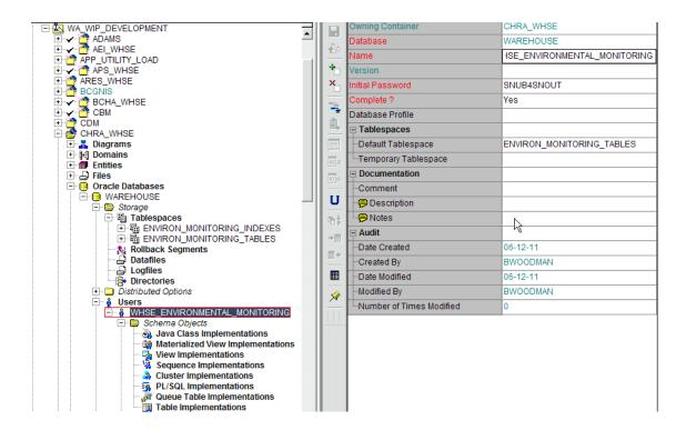
Once all the above conditions are met the physical model can be transformed from here. To transform the logical model to a physical model highlight the application container to be transformed, select the command "Database Design Transformer" located on the pull down menu Utilities  $\rightarrow$  Designer side menu. The Transformer starts:
