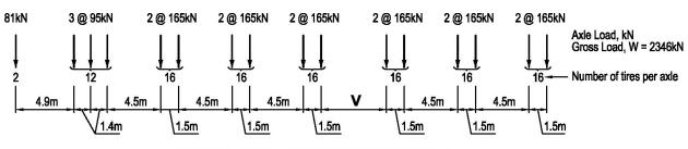
V = Variable Spacing - 4.5m to 18m inclusive. Spacing to be used is that which produces the maximum load effect.
