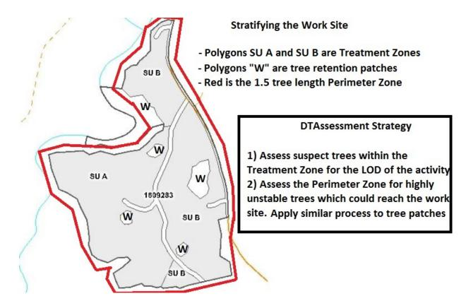
Figure 5: Example of a worksite stratified into tree assessment zones
