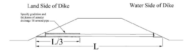
**Seepage collars (or anti-seepage rings)** – Assessment of past piping failures indicate that the presence of seepage collars often result in poorly compacted backfill<sup>4</sup> that can lead to dike failure and accordingly we do not accept the use of seepage collars as a means of preventing the migration of soils along the path of the pipe surface.
