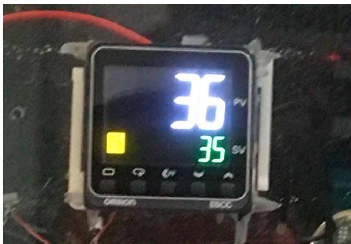
Figure 4. A display reads the ambient eRH (%) value in white (above) and target eRH (%) value in green.
