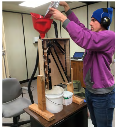
Figure 6. Air separation of debris and empty seeds using a zig-zag aspirator. Photo by Sybille Haeussler.
