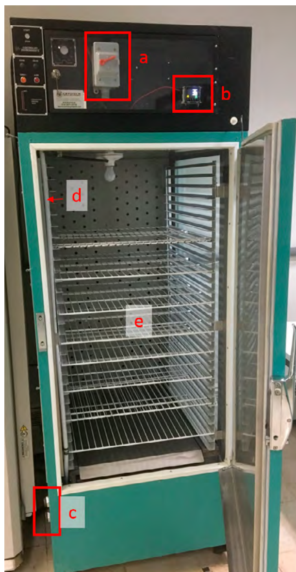
Figure. 1. The modified G30 Convicon chamber for use as an operational seed dryer, showing a) the power switch, b) display of the water activity in the chamber, c) outlets for humid air evacuation, d) location of the Omega HX71-MA water activity humidity probe and, e) new wire mesh shelving from Permafil.
