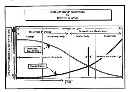
The owner must decide the best time to conduct one or more VE studies. Experience has shown that when two VE studies are performed, the first should be held at approximately the 15 percent stage and the second at about the 65 percent stage of the detailed design phase. If only one VE study is needed, the ideal time for conducting the VE workshop is at the 25 percent stage of design completion.
