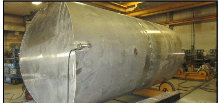
**PICTURED:** The custom-built 17,500-litre fish transport tanks to move fish from the concrete fish ladder to French Bar Creek.
