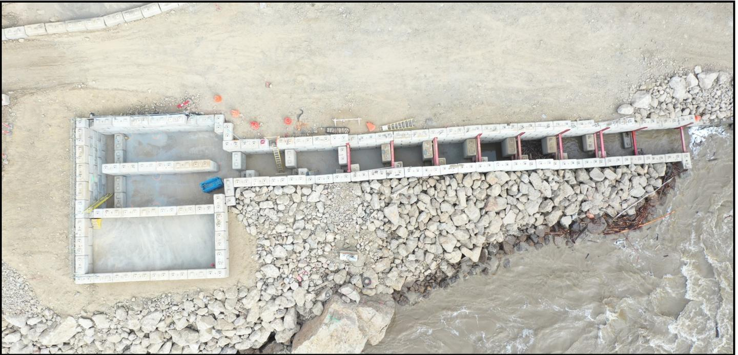
**TOP:** An aerial image of the concrete fish ladder; fish will swim up the ladder and into the holding area before being loaded into transport tanks for release upstream.
