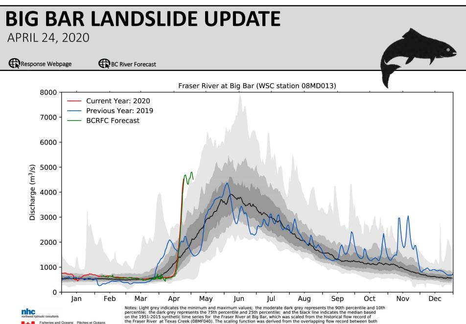
the Fraser River at Texas Creek (08MF040). The scaling function was derived from the overlapping flow record between both stations from 1951 to 1972. The current year represents observed flows at the Big Bar WSC gauge 08MD013. The forecasted flows are provided by the BC River Forecast Center
