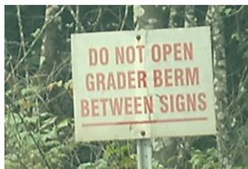
**Figure 14.** Big Tree Main south of the Jordon Junction in the Memekay watershed. This sign depicts a good example of a road-surface sediment management practice. Along this road section, a grader berm is maintained to allow sediment-laden water to flow past a stream before being directed without harm onto the forest floor.
