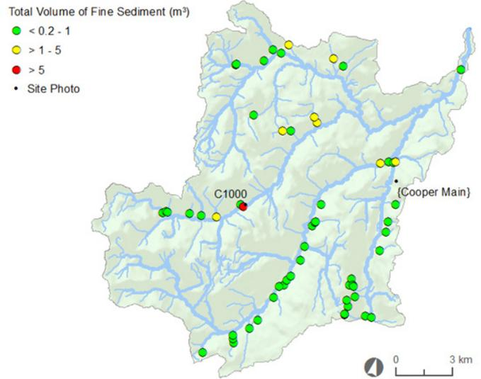
Figure 10. Sediment survey locations in the Memekay watershed, the sediment delivery rating at each site, and site identifiers for photos used in the report.
