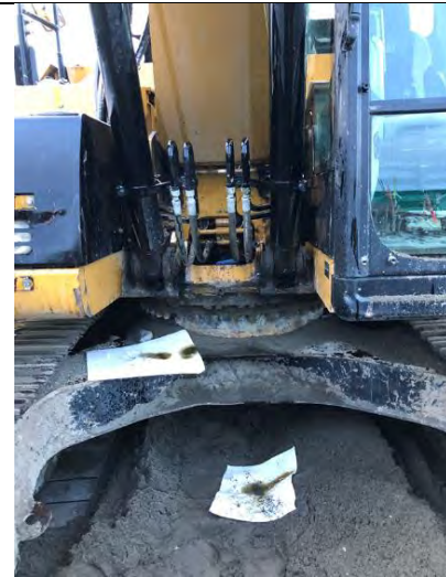
Photo 20. Hydraulic fluid from broken hydraulic line on excavator dripped onto machine and ground at the L500 (E).
