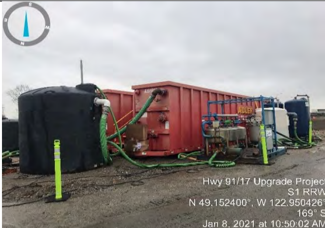
Photo 1. Stormtec water treatment facility for contaminated groundwater. System includes intake pumps, oxidation, pH adjustment, flocculation, settling tanks, and filters (C).
