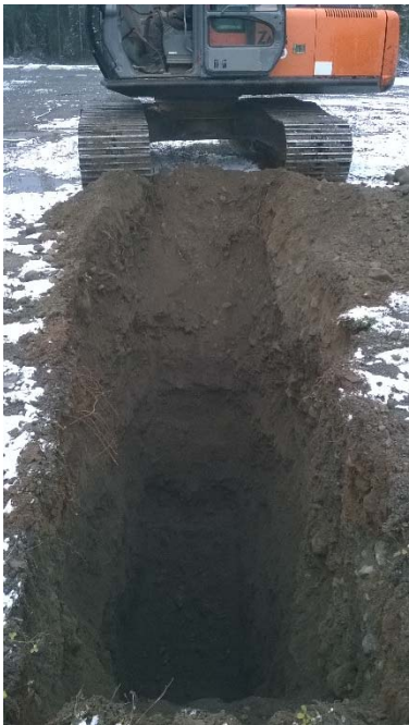
PHOTOGRAPH NO. 6: TP16-19 showing GP-GM soils typical for Area D.
