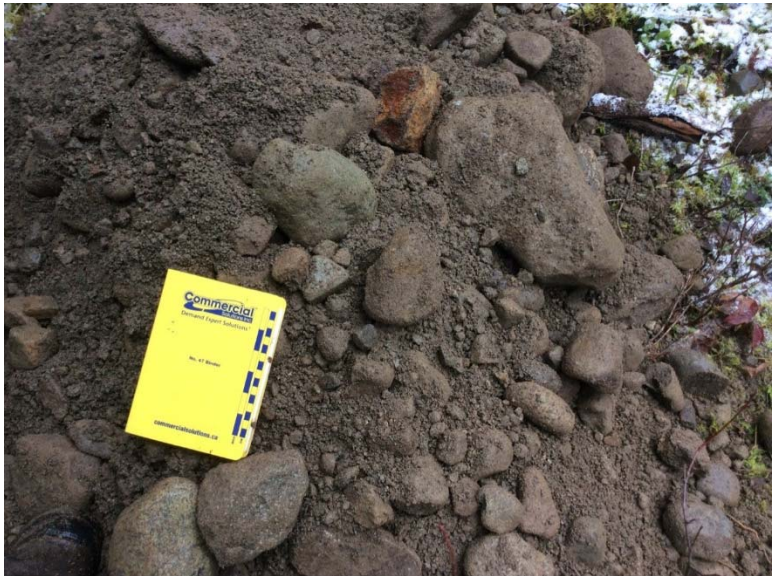
PHOTOGRAPH NO. 4: TP16-04 showing well-graded gravel with approximately 17% oversize material up to 300 mm diameter.
