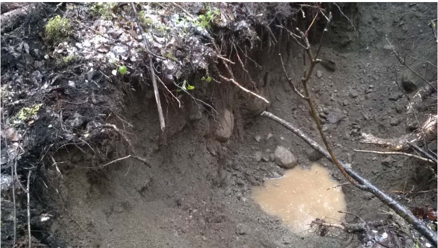
PHOTOGRAPH NO. 3: Water table encountered at approximately 2.2 meters depth in TP16-17.
