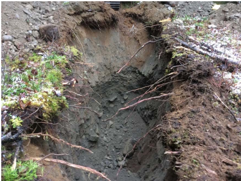
PHOTOGRAPH NO. 2: TP16-07 showing SW-SM to 1.2 m depth overlying GP soil typical for Area C.
