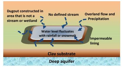
Figure 5. Dugouts containing only overland flow - no authorization reauired
