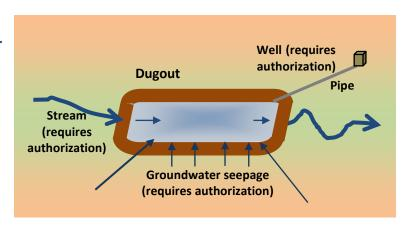
Figure 4. Mixed water supply dugout - authorization required
