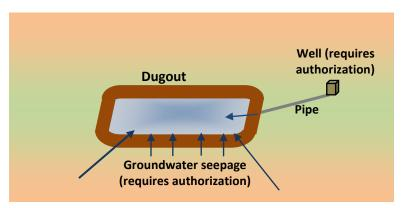
Figure 3. Dugouts diverting groundwater - authorization required
